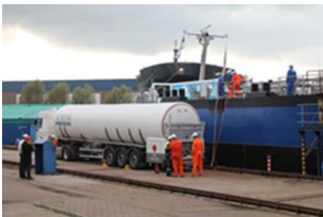
Mobile bunker location from tanker truck
